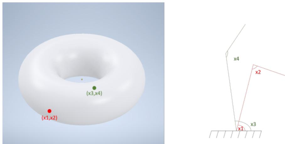
Figure 4: Torus and two robot positions
